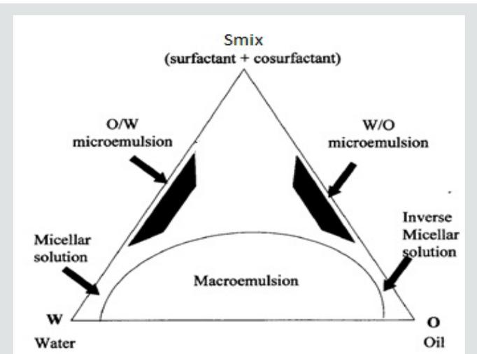
Figure 4: Phase diagram based on solubilisation theory.
