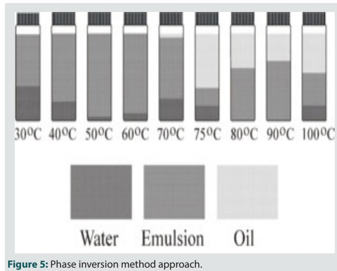
Figure 5: Phase inversion method approach.
