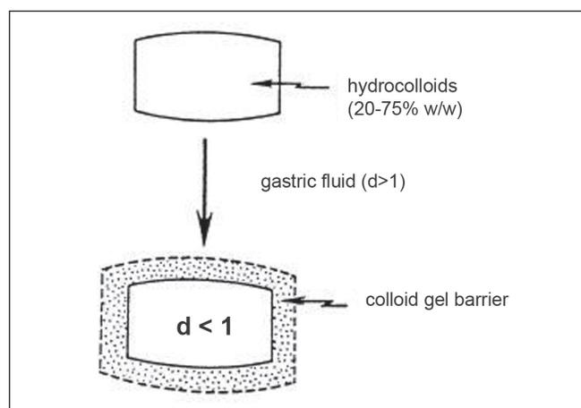
Figure 2: Intragastric floating tablet (US Patent 4, 167, 558, September 11, 1979)
