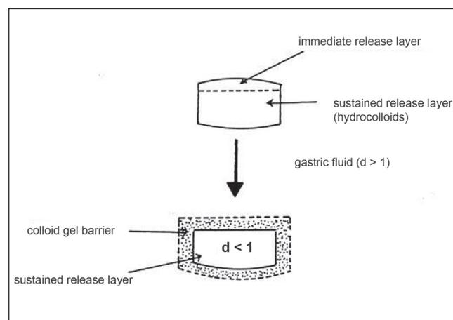
Figure 3: Intragastric floating bilayer tablet (US Patent 4, 140, 755, February 20, 1979)
