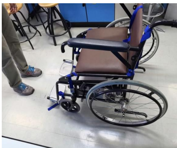
Figure 10: Test for stopping motion in front of human obstacles
