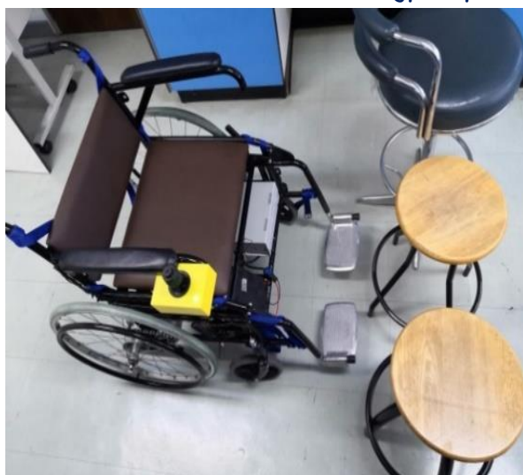
Figure 9: Test for stopping motion in front of loose structured obstacles
