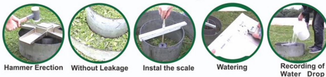
Figure 2: Instalation of double ring infiltrrometer.
