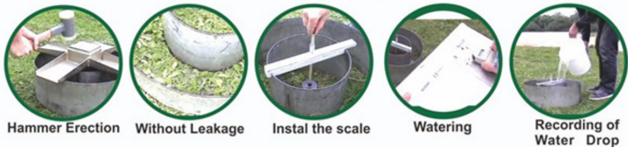
Figure 2: Instalation of double ring infiltrrometer.
