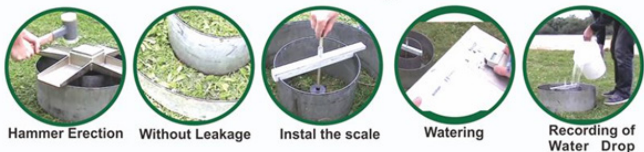
Figure 2: Instalation of double ring infiltrometer.
