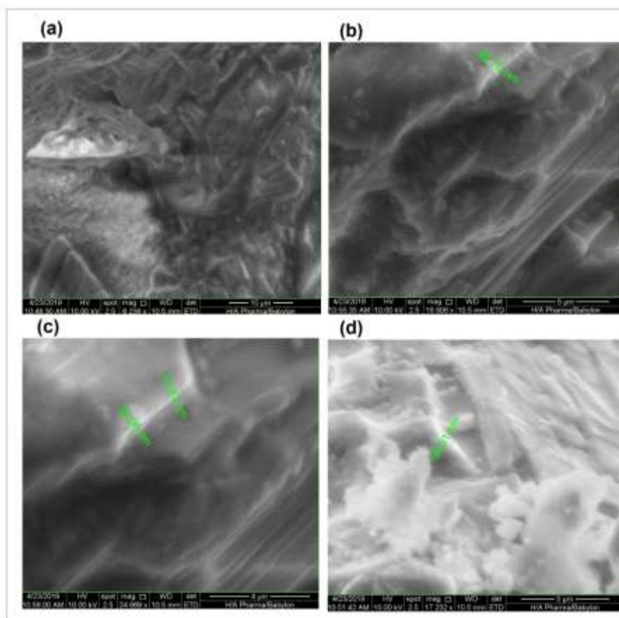
Figure 2: SEM of (a) synthesis CNTs, (b) Amino Functionalization of CNTs (c) (OH-COOH) Functionalization of CNTs, and (d) Loading of DOX on f-CNT
