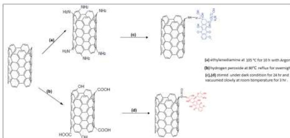
Figure 1: Functionalization of carbon nanotubes by two methods and loading DOX on CNTs
