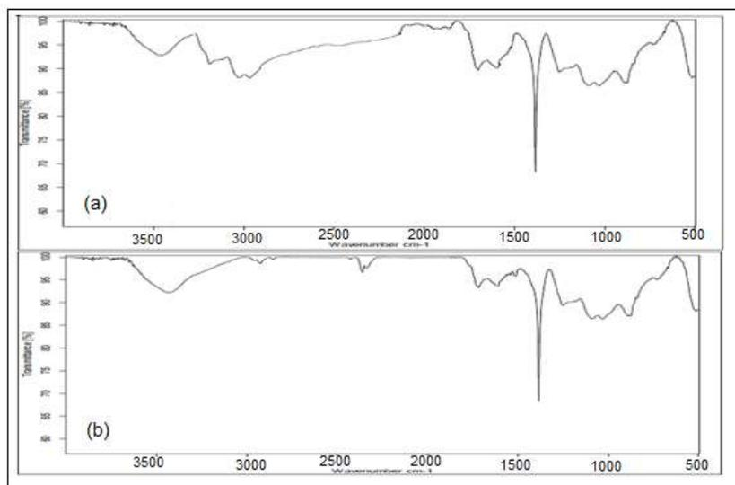
Figure 4: FTIR for (a) functionalized synthesized CNTs ( $\text{-NH}_2$ ), and (b) functionalized synthesized CNTs ( $\text{-OH}$ ,  $\text{COOH}$ )
