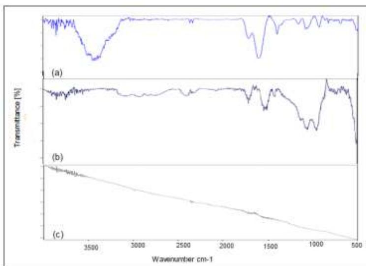
Figure 3: FTIR for synthesized CNTs (a) before purification, (b) after Purification by H<sub>2</sub>O<sub>2</sub>, and (c) after purification by (H<sub>2</sub>O<sub>2</sub>), acetone, calcined at 500 °C for 2 h
