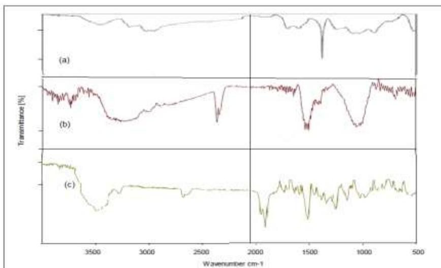
Figure 7: FTIR (a) functionalized synthesized CNTs (-NH), FTIR for Doxorubicin drug, and FTIR for loading Doxorubicin drug on N- CNTs.
