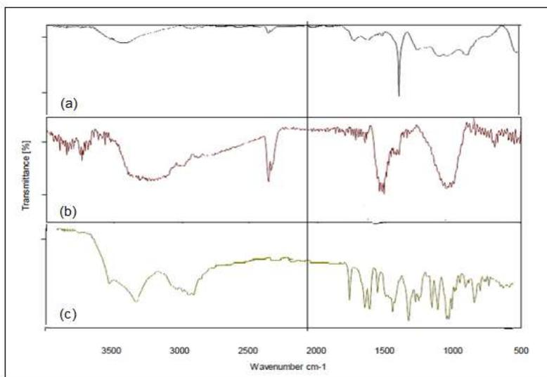
Figure 6: FTIR (a) functionalized synthesized CNTs (-OH, -COOH), FTIR for Doxorubicin drug, and FTIR for loading Doxorubicin drug on O- CNTs.
