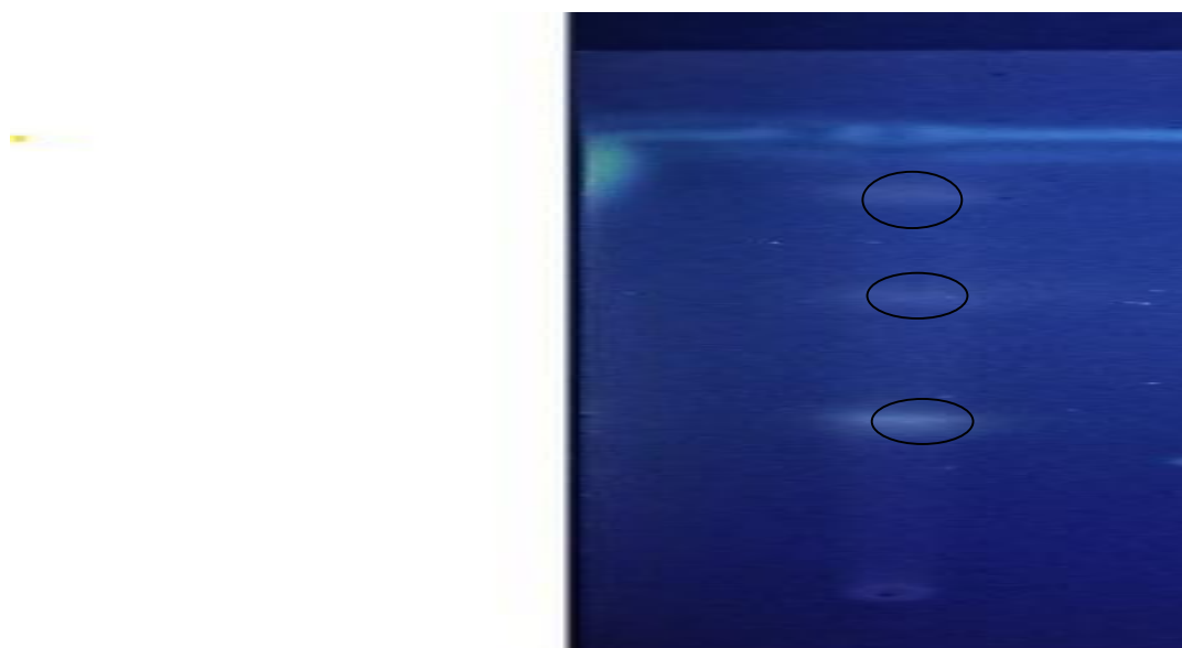
Figure 1: UV visualization of 366 nm results from TLC of ethyl acetate fraction using hexane: ethyl acetate: formic acid (6: 4: 0.2) solvent
