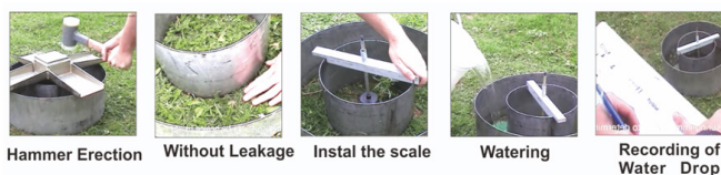
Figure 1 B: Installation of double ring infiltrometer
