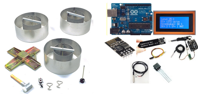
Figure 1 A: Double ring infiltrometer and sensors
