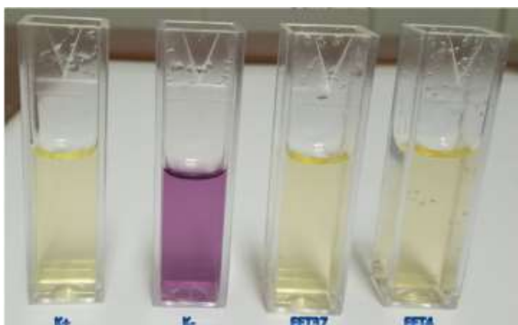
Figure 2: Antioxidant testing via the DPPH method. The ability of hydrogen atom donors causes purple to yellow discoloration obtained in the groups of vitamin C (K+), Curcuma Ethanol Extract stored at 37 °C (EET37), Curcuma Ethanol Extract was stored at 4 °C and purple blanks (K-).
