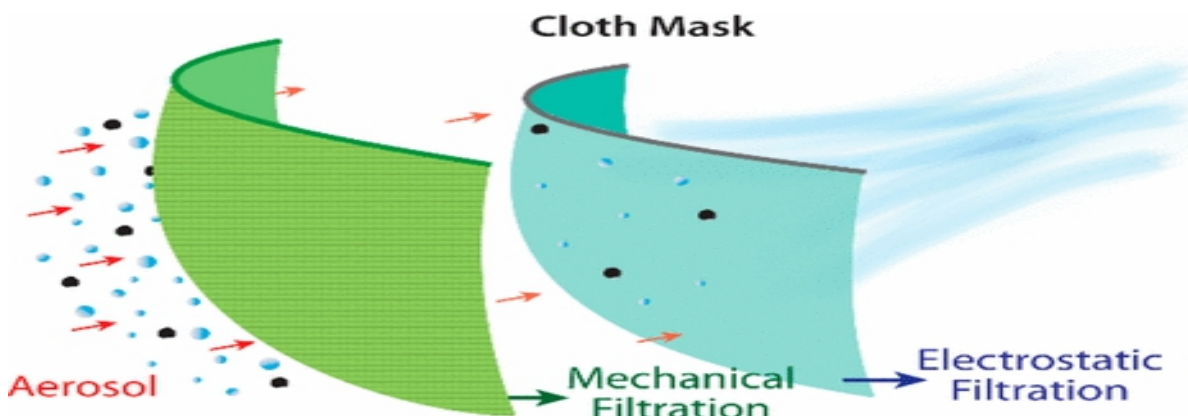
Figure 3. The process of aerosol filtration of a cloth mask (38).
