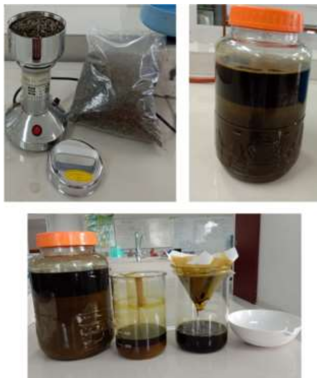
Figure 1: Production of EGCG in East Javanese green tea using maceration method.
