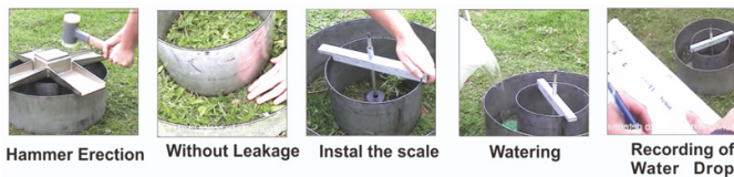
Figure 1B: Installation of double ring infiltrometer
