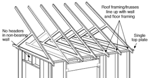
Figure 2: Advancement Framing on In-Line
