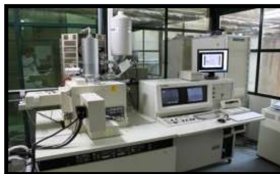
Figure 1: Scanning Electron Microscope (Field Emission SEM, S-4160, HITACHI, Tokyo, JAPAN)
