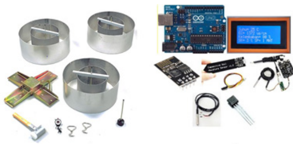
Figure 1A: Double ring infiltrometer and sensors
