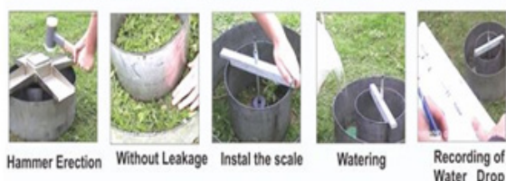
Figure 1B: Instalation of double ring infiltrator
