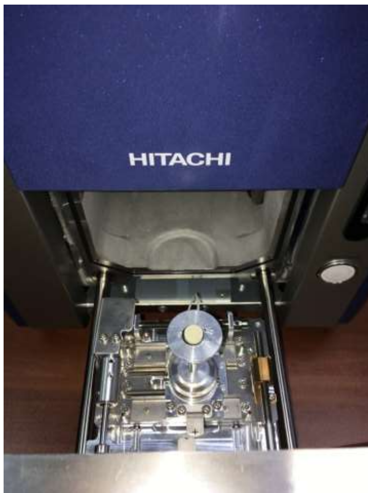
Figure 3. Stage of installation of the stage with an experimental titanium implant with the Bioactive Covering on the Basis of Synthetic Complex with Biogenic Elements
