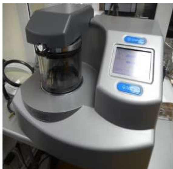
Figure 1. Photo. Quorum Q150 ES Vacuum Post and Process Preparation of a procedure for spraying a conductive layer with a piece of bone tissue to form a conductive layer and further study in an IR spectrometer.
