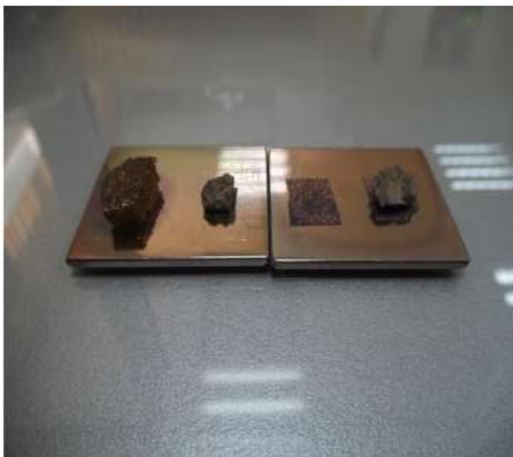
Figure 2. The result of the deposition of a conductive layer on the surface of the bone tissue
