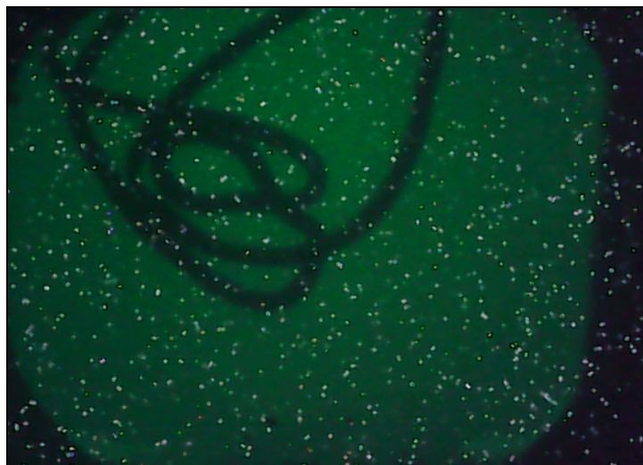
Figure 4: noise effecting on image due to x-ray leakage
