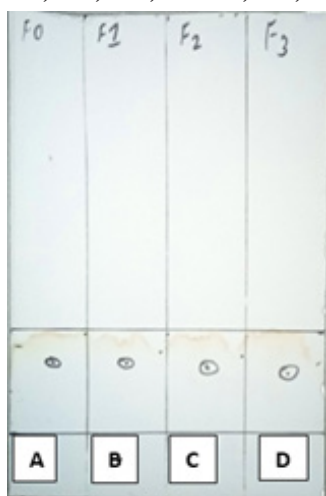
Figure 1: Silica gel plate chromatography; (A) Fraction 0 (F0) the very first elute of the extract which was subjected to column chromatography, (B) Fraction 1 (F1) second elute of the extract which was subjected to column chromatography, (C) Fraction 2 (F2) third elute of the extract which was subjected to column chromatography, (D) Fraction 3 (F3) third elute of the extract which was subjected to column chromatography
