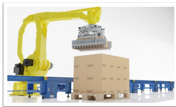
Figure 5: Palletizing robots in the task of packing finished products
